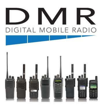
Digital mobile radio (DMR) is an open digital mobile radio standard defined in the European Telecommunications Standards Institute (ETSI) Standard TS 102 361.
