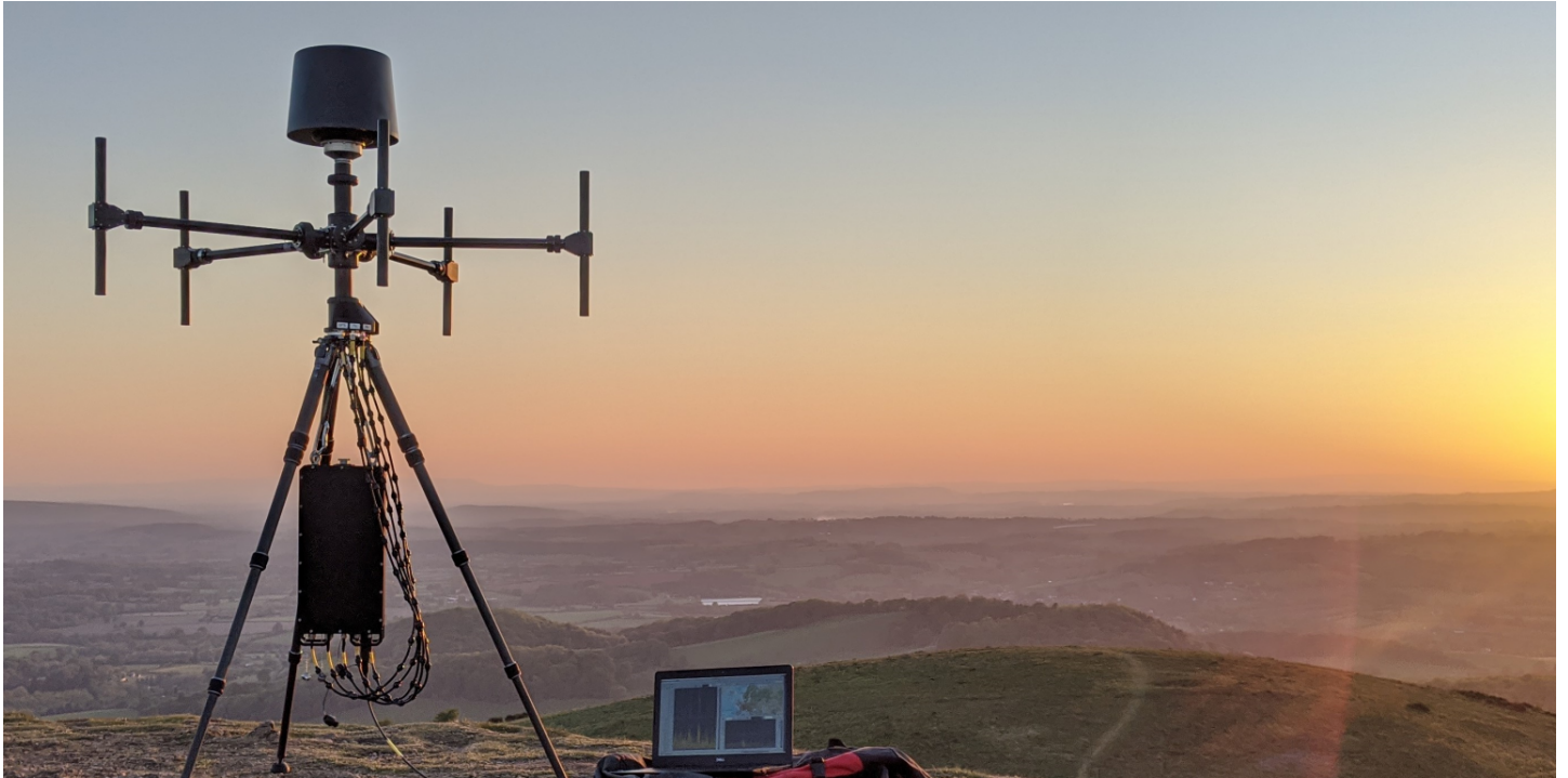
CommsAudit’s dismounted EW systems include the Spectra Go tactical DF unit which covers a 30MHz to 6GHz waveband. (Photo: CommsAudit)
